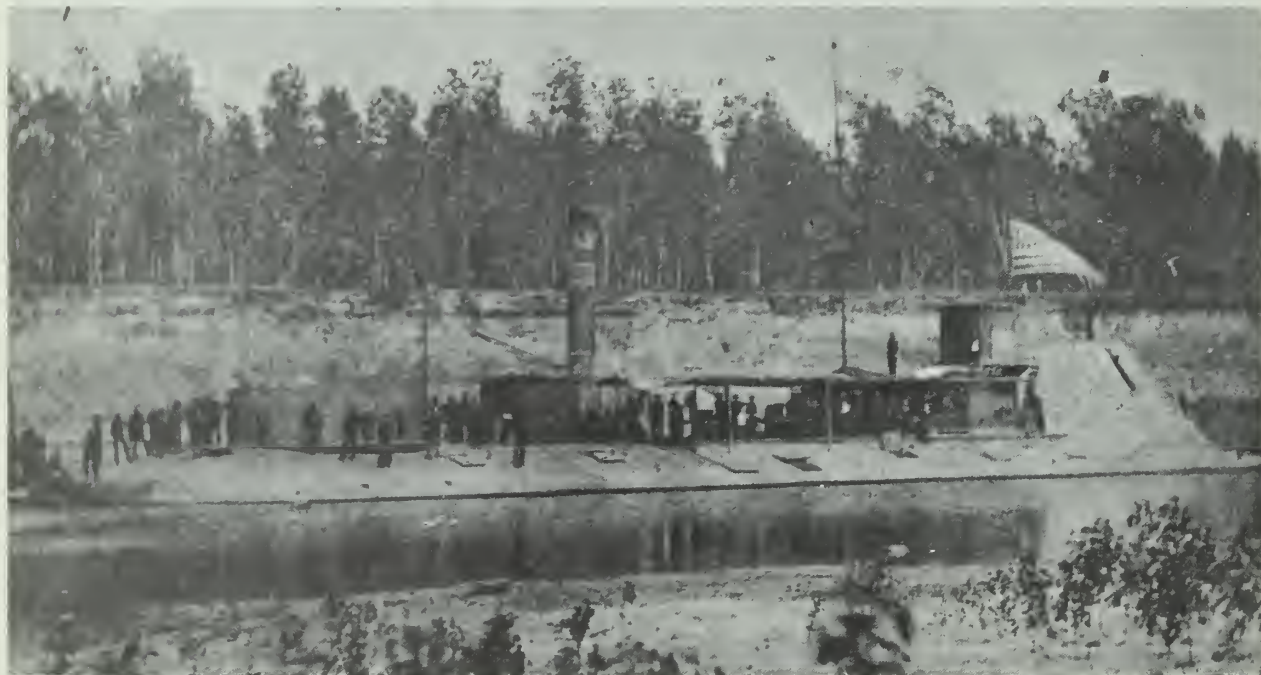
USS Osage shown on the Red River during the 1864 expedition in support of General Banks—Additional deck structures erected since the previous photograph can be seen. Thomas O. Selfridge, Jr., who commanded USS Osage at this time, spoke in his memoirs of using a periscope mounted on the turret to direct fire of the battery.
